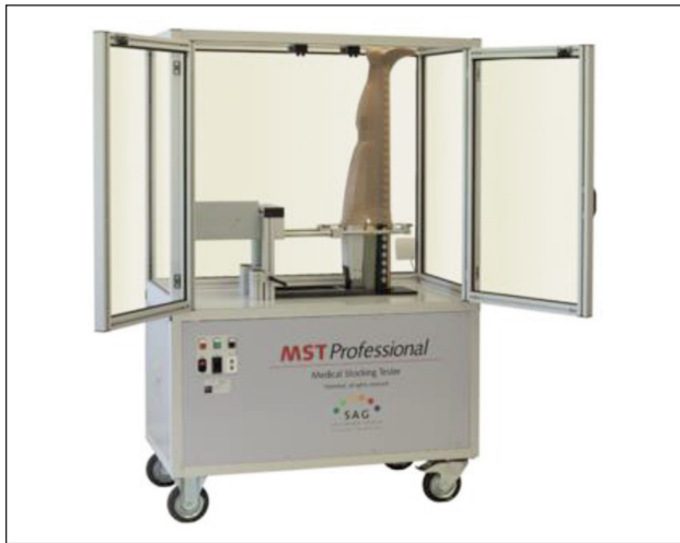
Fig. 5. MST Professional II medical stocking tester
